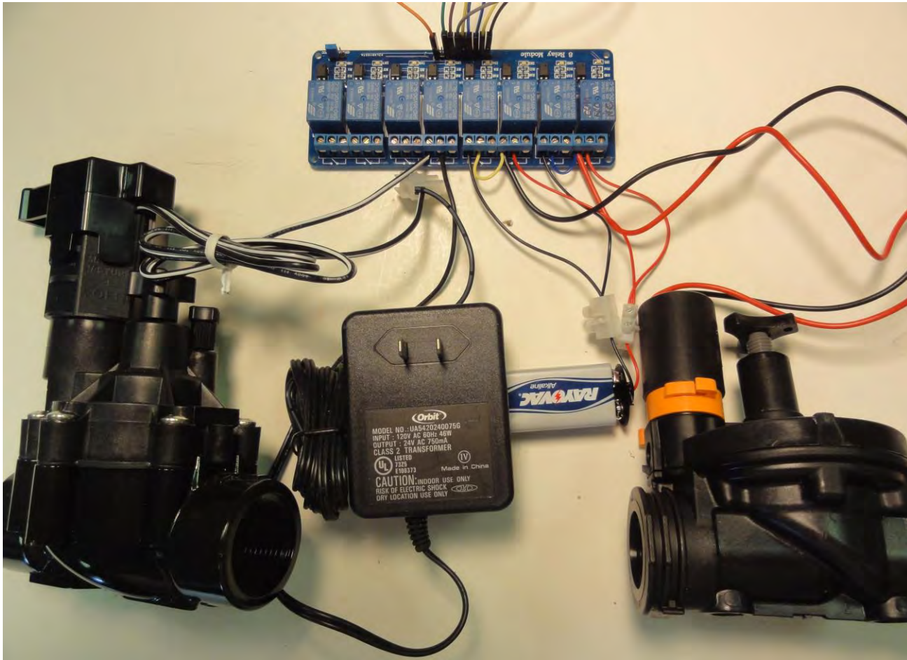
View of one latching and one regular solenoid valves connected to relays
