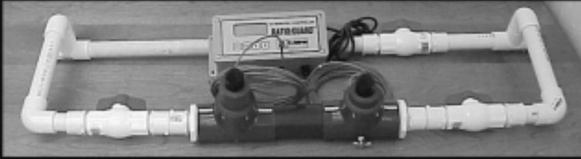
Figure 5. An EC meter can be installed in your water line to continuously monitor the electrical conductivity of your water or fertilizer solution. This is a very simple way to make sure that you are applying the correct fertilizer concentrations to your crop.
