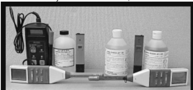
Figure 1. To measure the EC and pH of your fertilizer solution on growing medium, you will need an EC meter, a pH meter and three calibration solutions (one for the EC meter and two for the pH meter)
